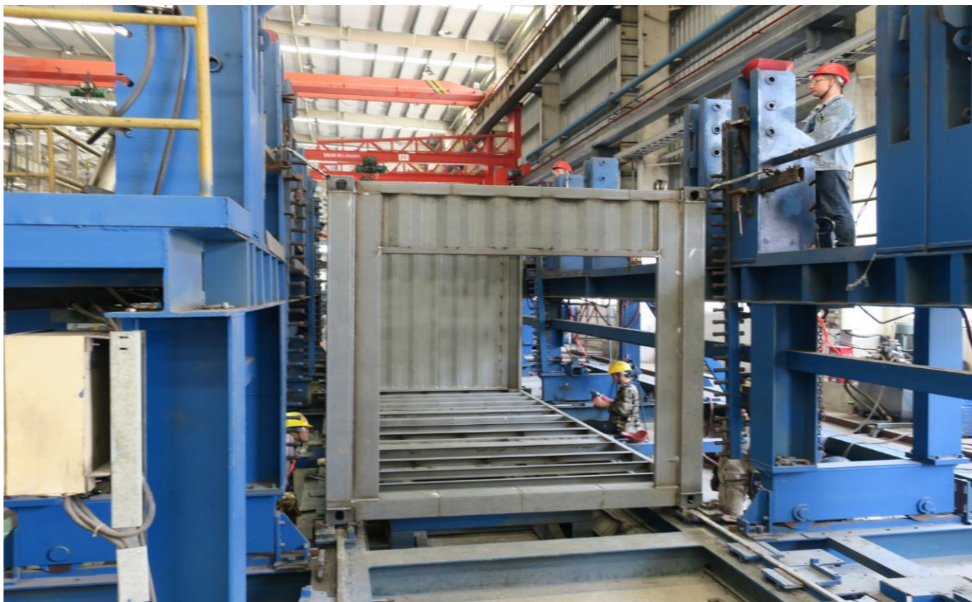
Modules being machined and hand welded within the manufacturing jig
